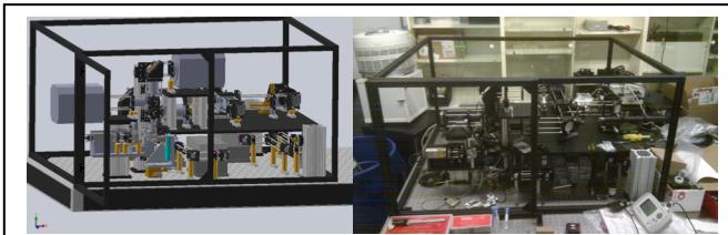
Fig. 2: Connectoscope V1 based on RESOLFT.
