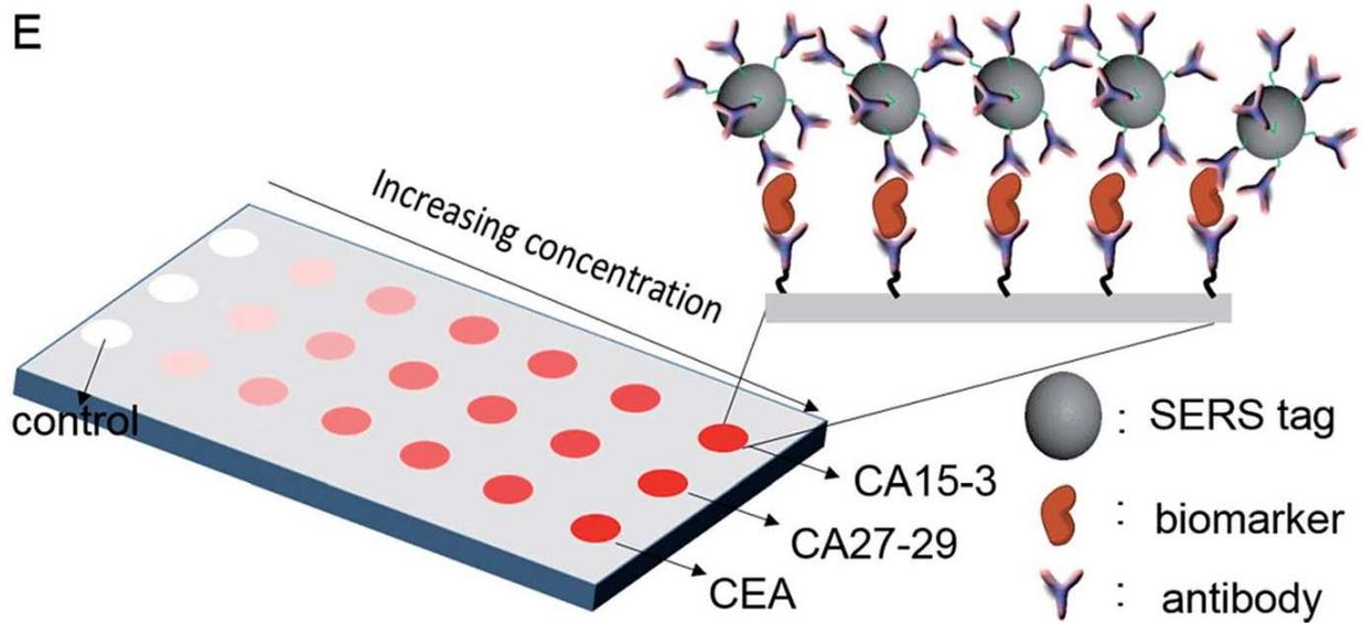
Schematic illustration of SERS assay for multiplex detection of biomarkers
